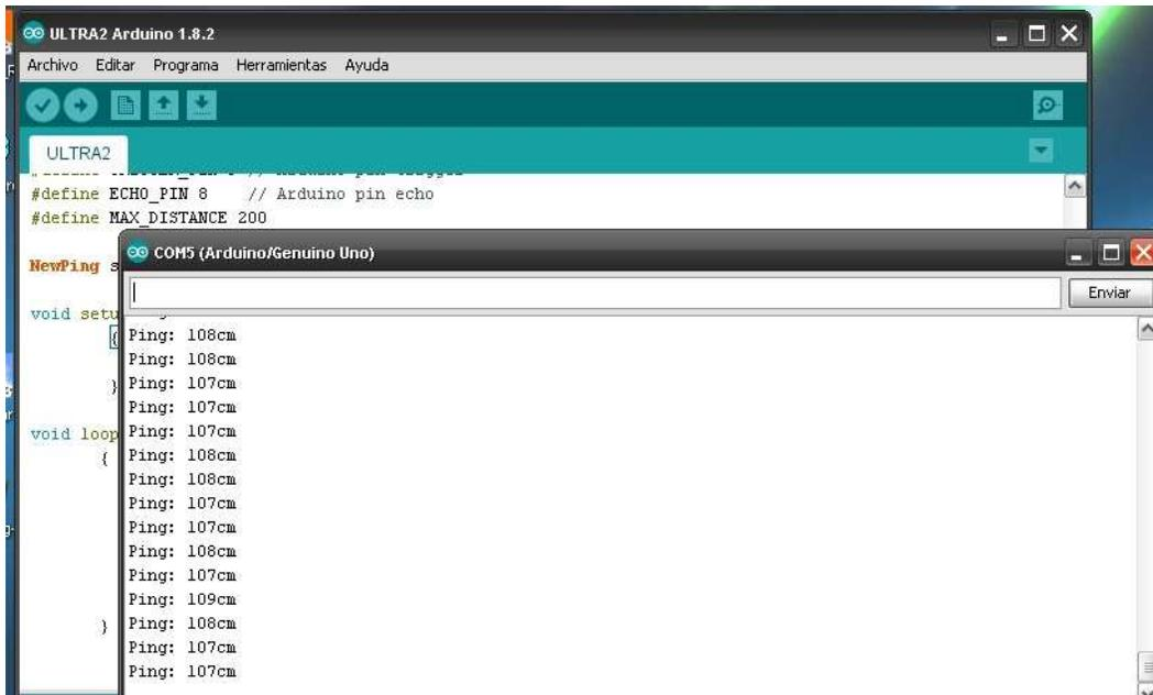
The screenshot shows the Arduino IDE interface. The top window displays the code for the NewPing library example. The serial monitor window, titled 'COM5 (Arduino/Genuino Uno)', shows the output of the program, which consists of a series of 'Ping: [distance]cm' messages. The distances alternate between 108cm and 107cm, with one instance of 109cm.
